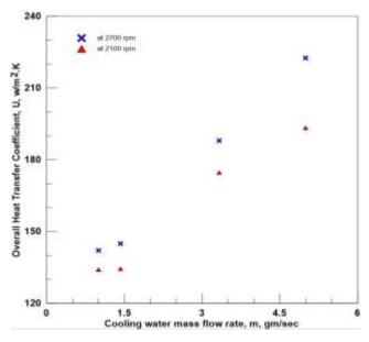
Figure. 11. Overall heat transfer coefficient at different cooling rates for FR=50% benzene at different engine speeds.
