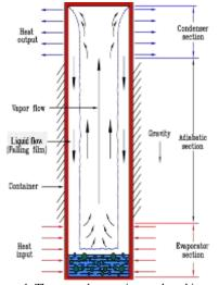
Figure 1. Thermosyphon sections and working principle
