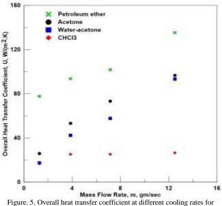
Figure. 5. Overall heat transfer coefficient at different cooling rates for FR=25% different working fluids at 1400rpm.
