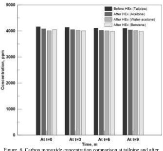
Figure. 6. Carbon monoxide concentration comparison at tailpipe and after heat exchanger charged with FR=25% of various working fluids at 1400 rpm
